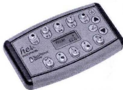
Figure 6.3 Tech Patient ECG Simulator [17]
