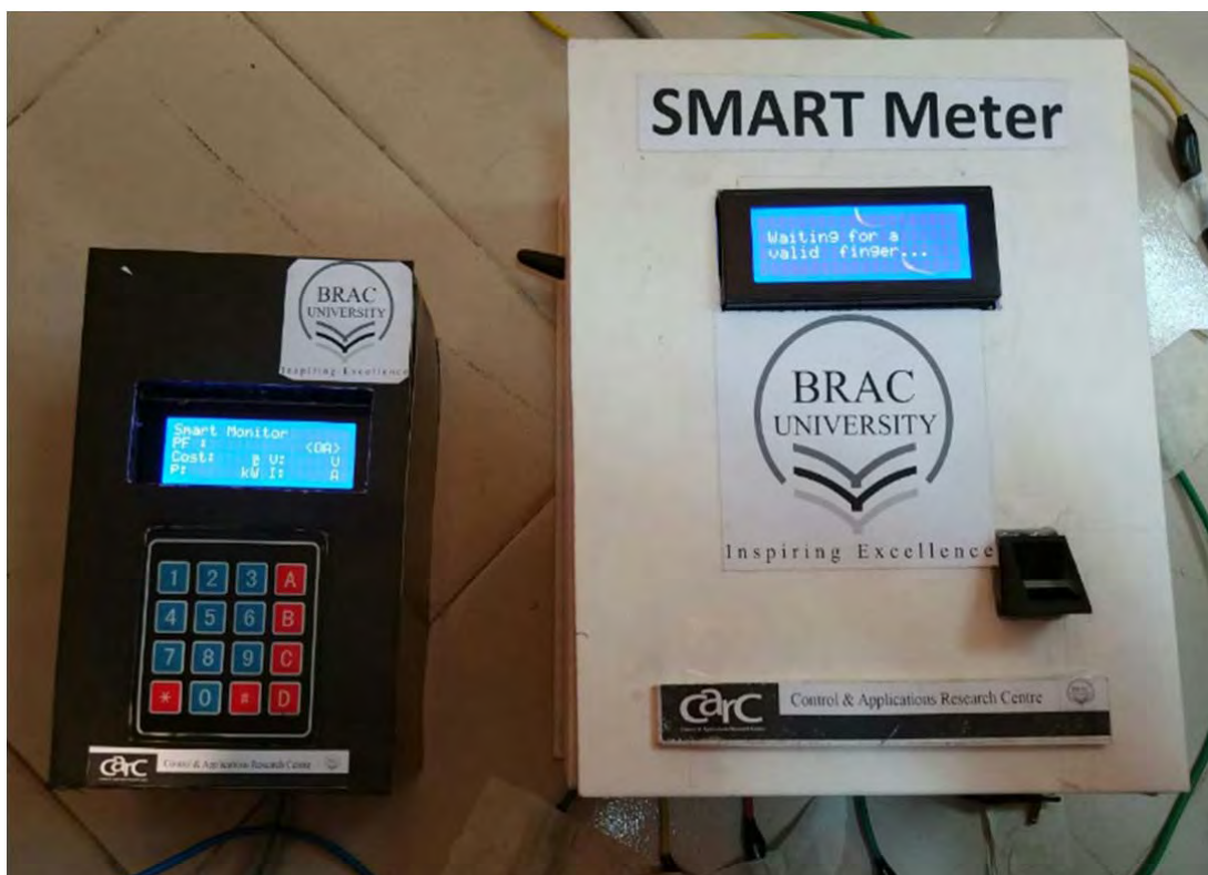
Figure 5.2: Secondary Monitor (Left One) and Main Meter Monitor (Right One)
