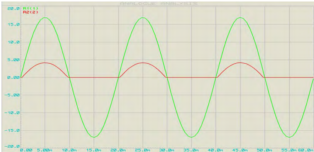
Figure 3.7: Optocoupler circuit Input and Output Voltage Graph
