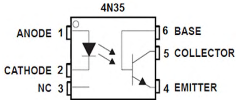
Figure 3.4: Optocoupler Pin Configuration [13]
