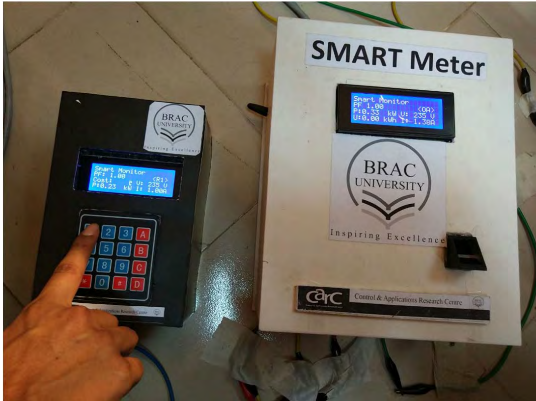
Figure 7.5: Getting Electricity Consumption for Room1 from Meter
