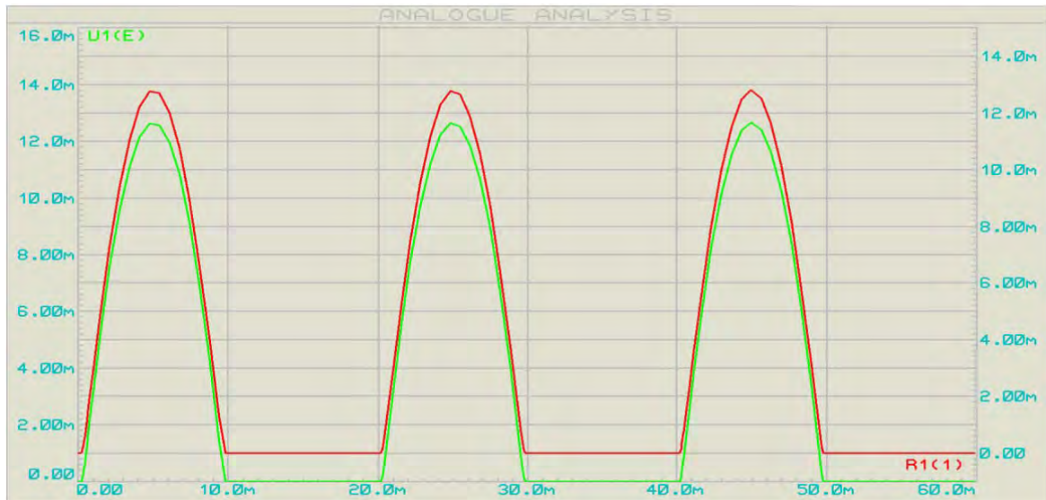
Figure 3.6: Optocoupler circuit Input and Output Current
