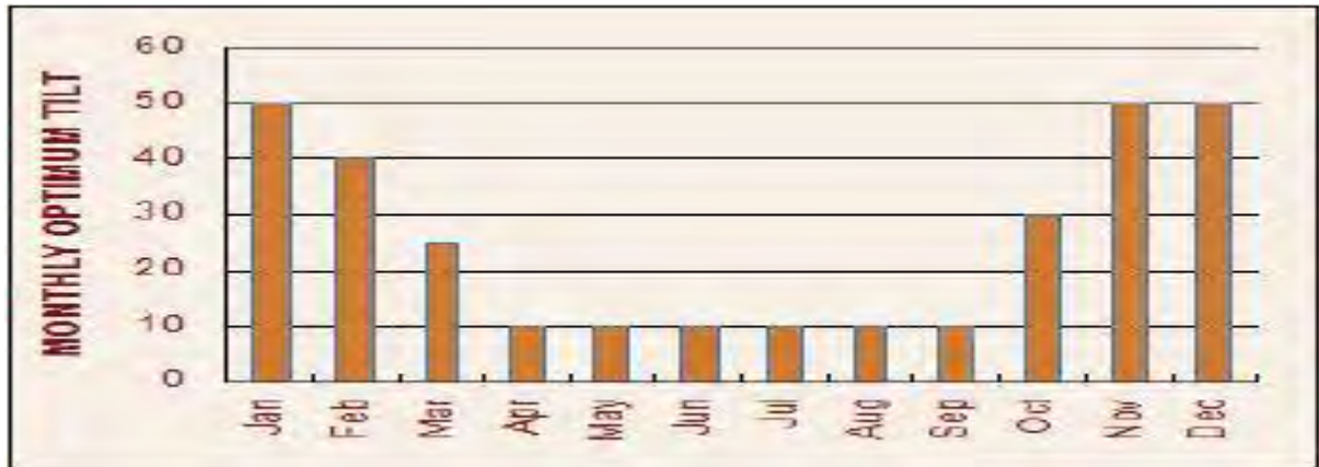
Figure 5.16 Optimum tilt for different months of the year [89]
