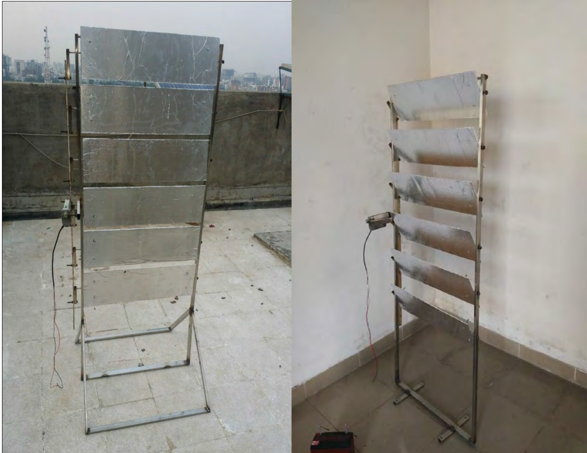
Fig 2.16: Solar panel Reflector
