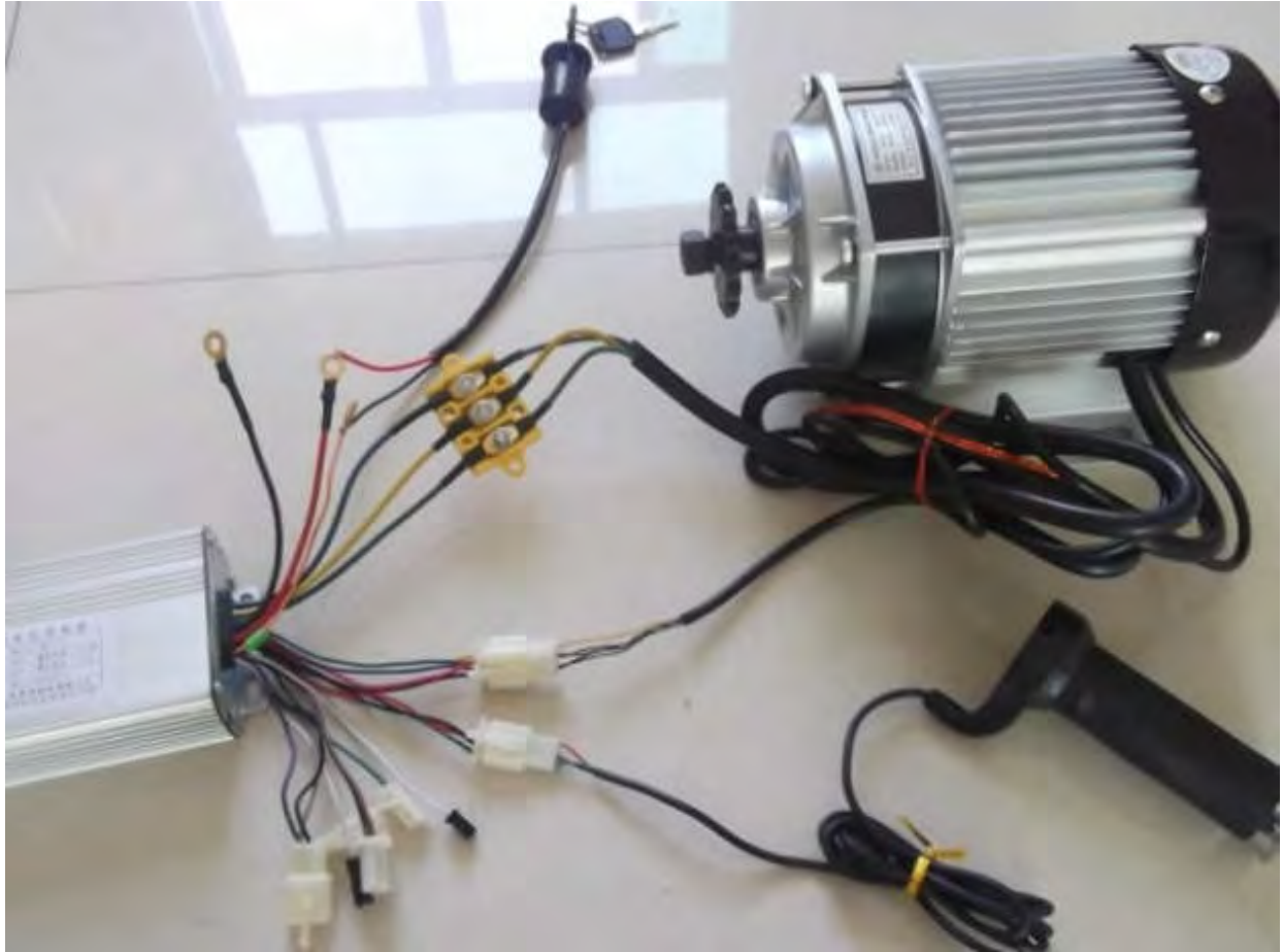
Figure 2.4 The Motor Controller Unit Connections
