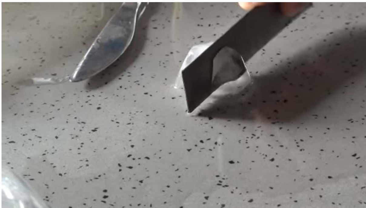
Fig: 4 (b) Using a graphene strip to cut through ice
