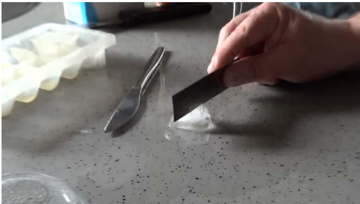
Fig: 4 (b) Using a graphene strip to cut through ice
