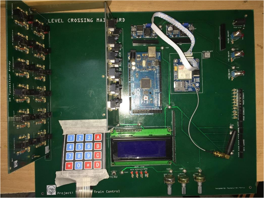
Figure 7.13 Level Crossing Mainboard
