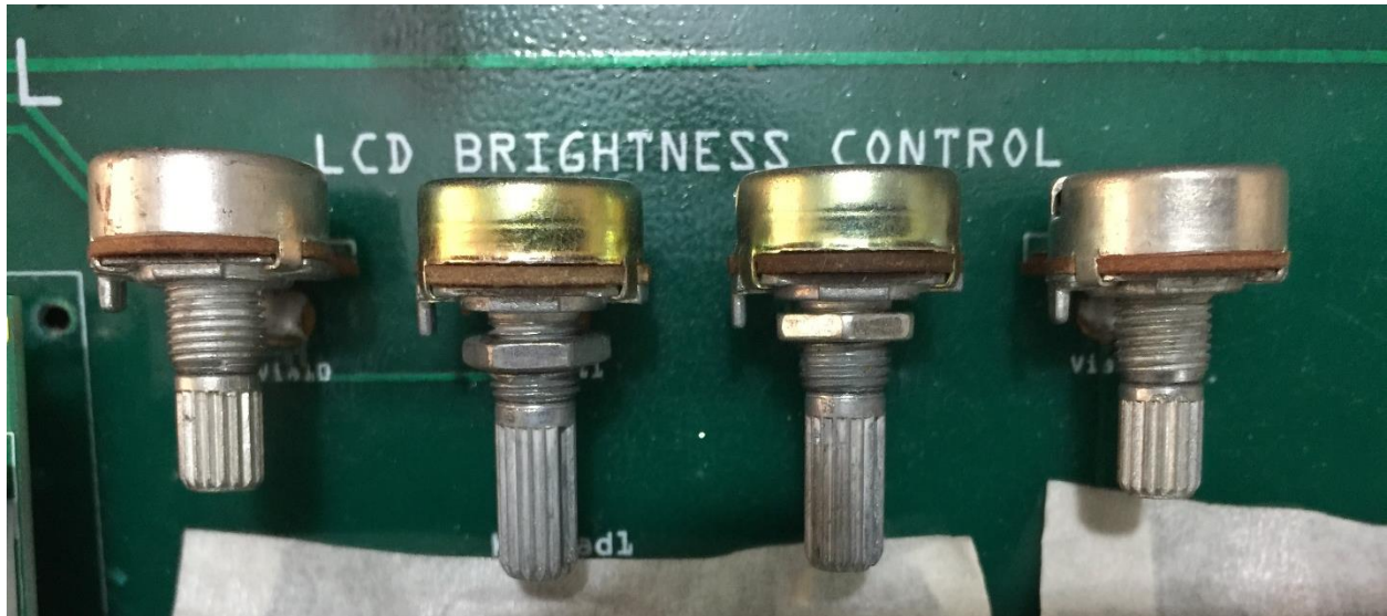
Figure 6.14 Potentiometers to Control LCD Brightness
