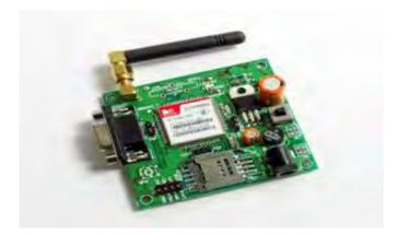
Figure 3.5: GSM Module
