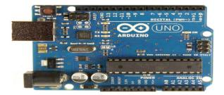
Figure 3.1: Arduino R3 Board
