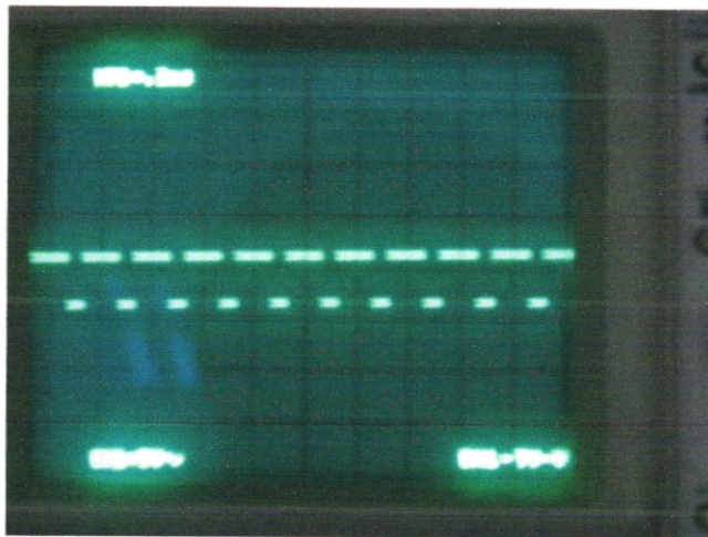
Figure15: When the voltage of battery is at 13.8V is switches to the absorption state of charging. In this state the PWM duty cycle is reduced to 70% of the total duration, i.e. 70% on.
