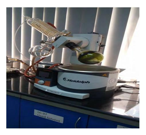
Figure 2.2: Concentrating the filtrate of A.scaphula plant using a rotary evaporator.
