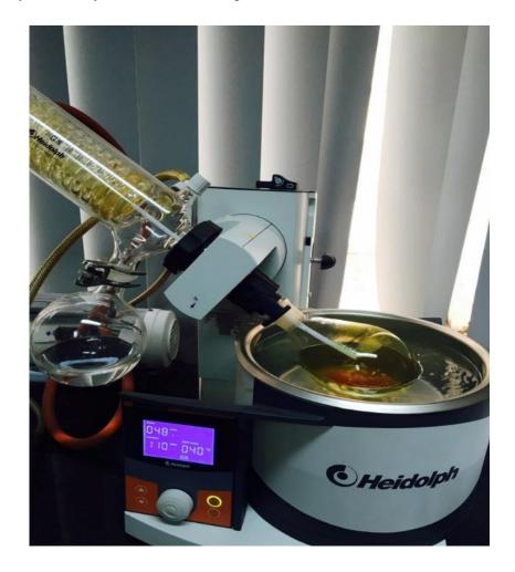
Figure 3.1 Rotary vacuum evaporator
