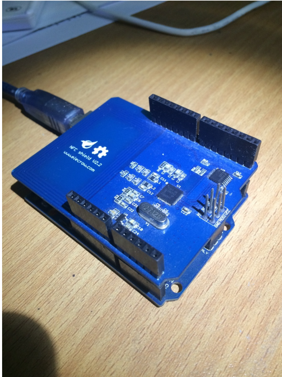
Fig.6.13. NFC connected to arduino
