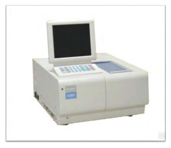
Figure 2.2: UV Spectrophotometer
