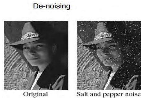
Figure 2.6: Linear filtering “salt and pepper” noise [12]
