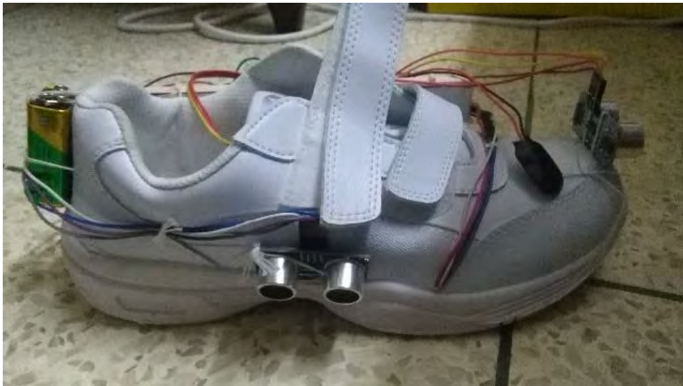
Figure 47 The right shoe with the ultrasonic sensor at the right side
