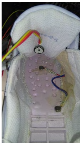
Figure 44 The pulse rate sensor under the flap and the vibration motors on the sole of the right shoe
