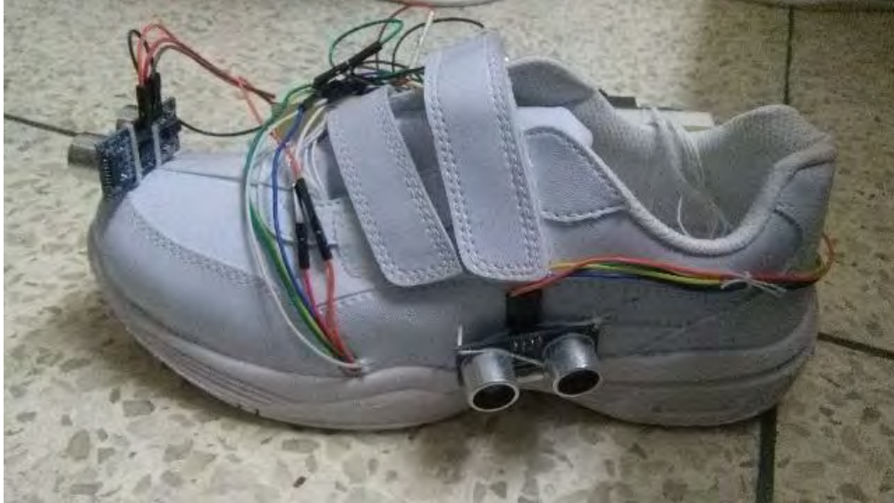
Figure 46 The left shoe with the ultrasonic sensor at the left side
