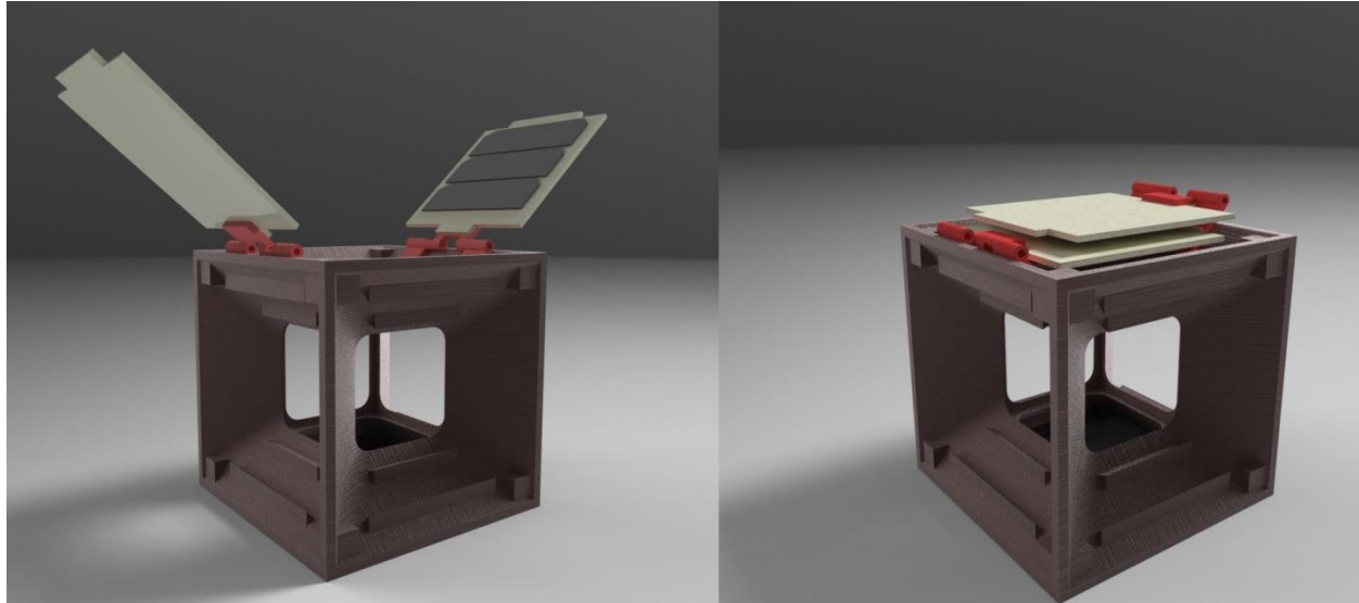
Figure 3: Solar panels in un-deployed and deployed position
