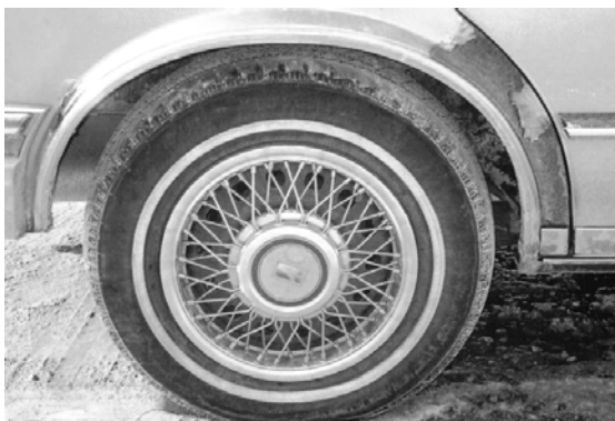
Figure 3: Galvanic corrosion on a car.
