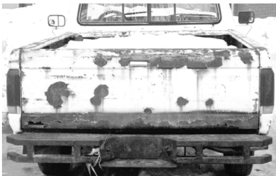
Figure 5: Pitting corrosion on a pickup car.
