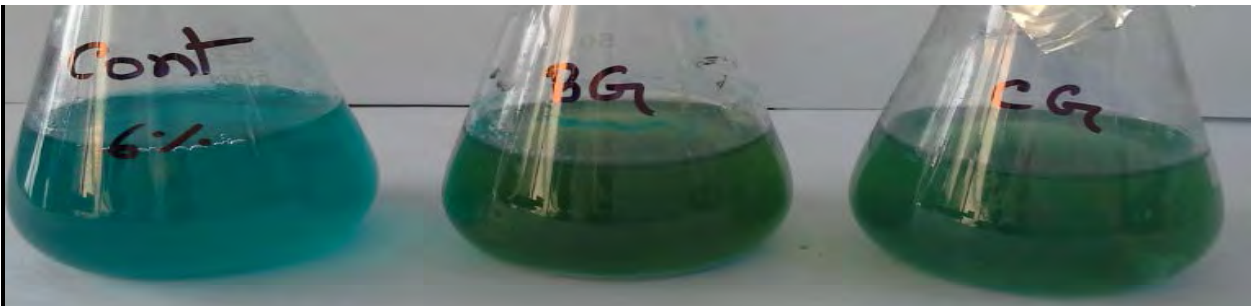
Figure 3.3.3 (III): Effect of 6% NaCl on decolourization of the GGS dye by isolates BG and CG when incubated for 5 days at 37 0 C.
