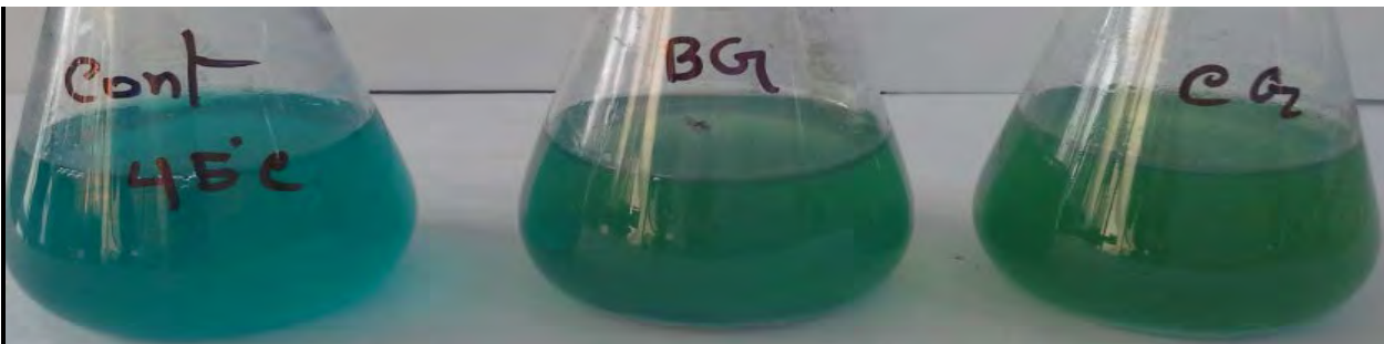
Figure 3.3.4 (III): Effect of 45 0 C on decolourization of the GGS dye by isolates BG and CG when incubated for 5 days.
