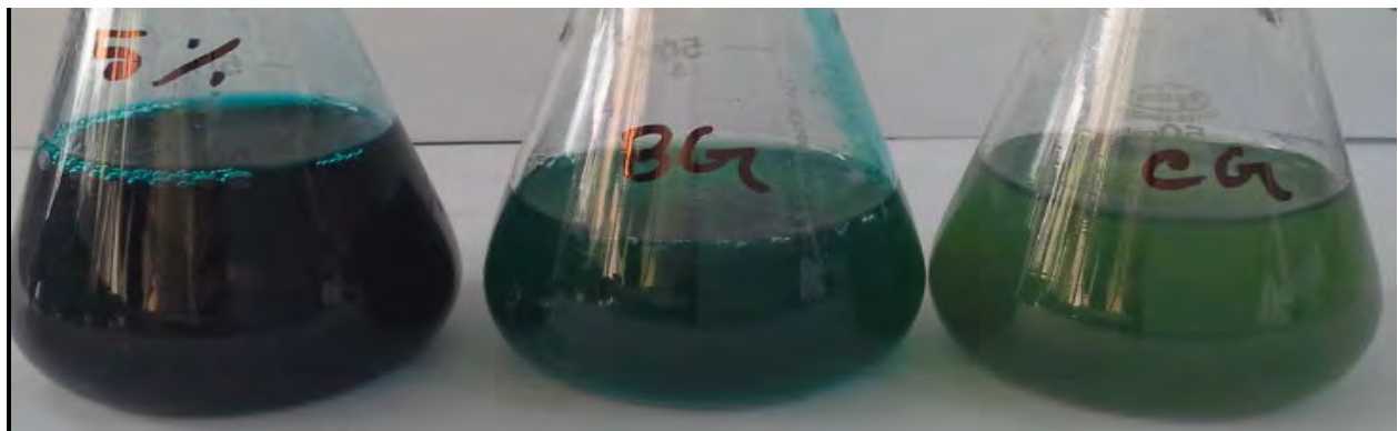
Figure 3.3.1(iii): Decolourization of GGS dye at 5% dye concentration by the isolates BG and CG when incubated for 5 days at 37 0 C
