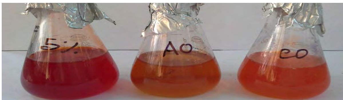
Figure 3.2.1(III): Decolourization of OM2R at 5% dye concentration by the isolates AO and CO when incubated for 5 days at 37 0 C.
