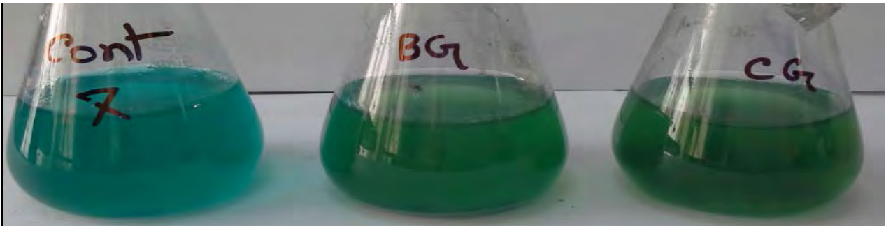
Figure 3.3.2 (III): Effect of pH 7 on decolourization of the GGS dye by isolates BG and CG when incubated for 5 days at 37 o C.
