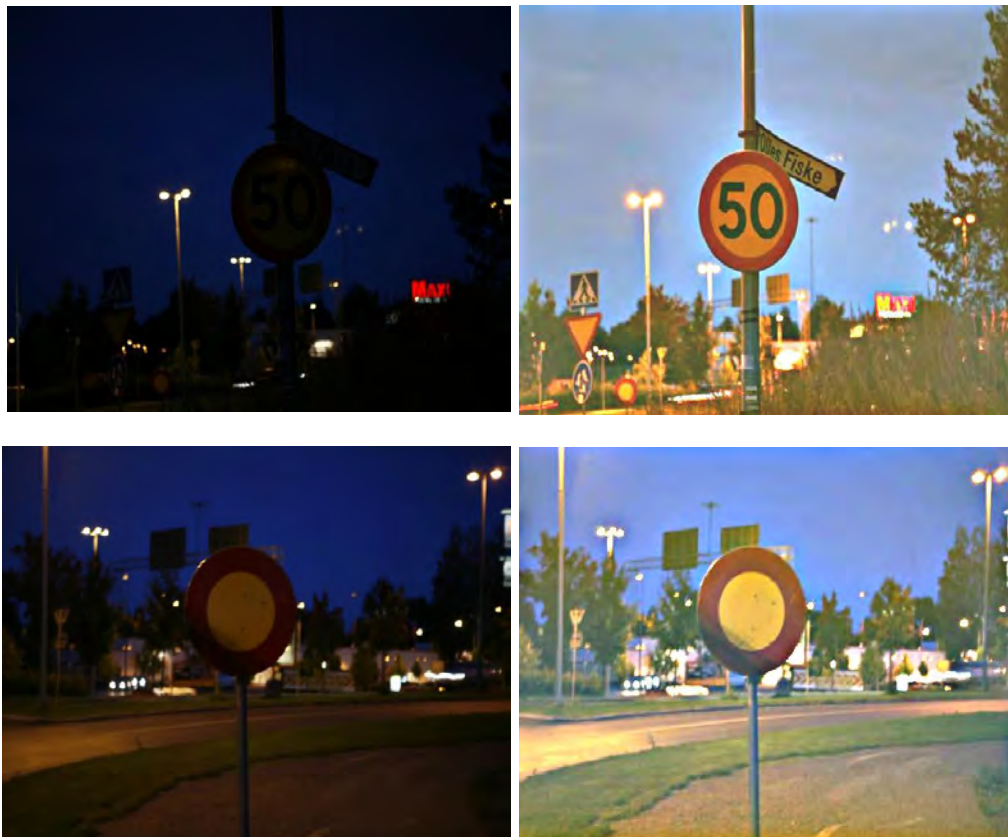
Figure-4.2.1.1: Before and After Applying MSRCR [9]
