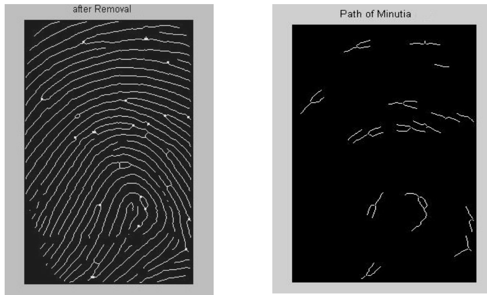
Fig 6.1.4: Fingerprint Image after removing false Bifurcations (Left Side), Showing the Path of the Minutiae (Right Side)
