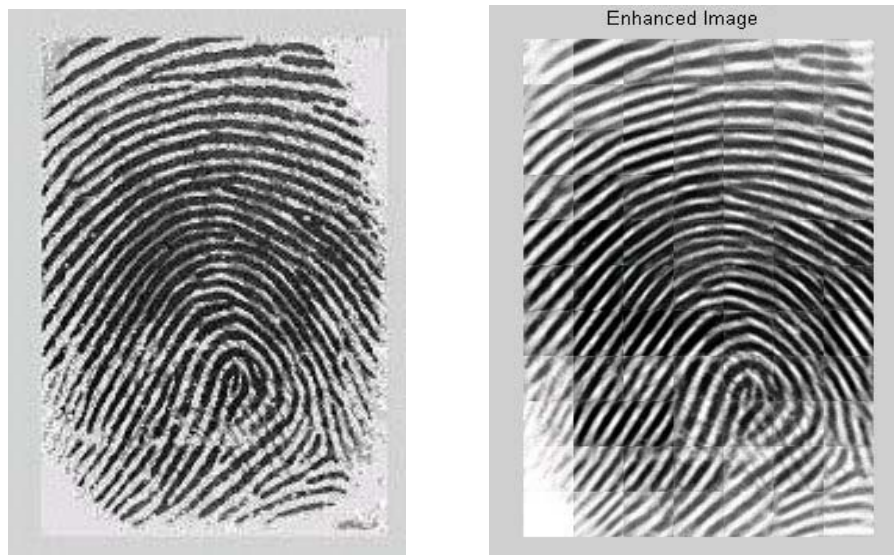
Fig 4.1.3: Image enhancement by Histogram Equalization (left side), Image enhancement by FFT (right side)
