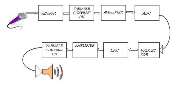
FIGURE 2.1: Block Diagram Of The Sysytem
