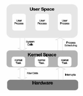
FIGURE 3.1: Operating System Architecture
