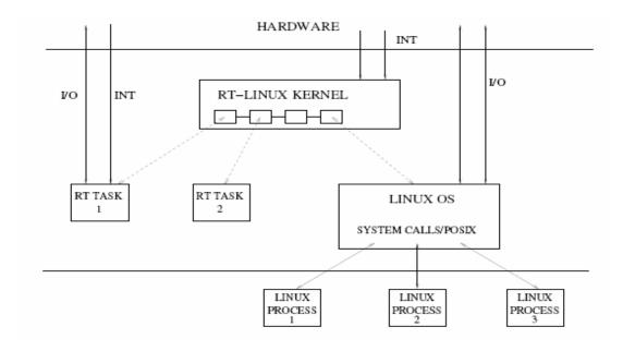
FIGURE 3.2: RT-Linux System Structure
