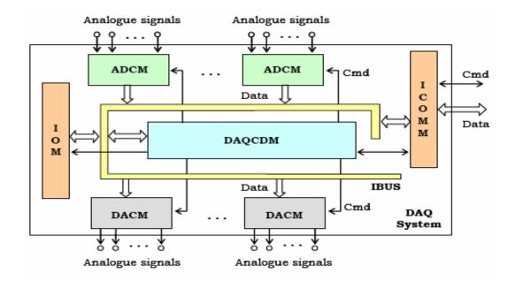
FIGURE 3.3: DAQ Architecture
