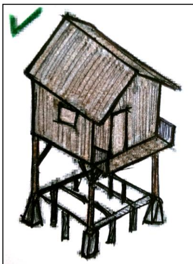
Fig 4. 48: Construction on silts Source: Prepared by author from IFRC (2011)
