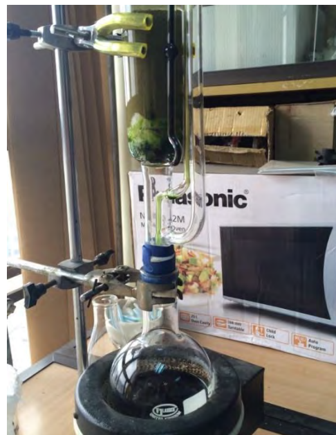
Fig 1: Extract collection through Soxhlet Apparatus
