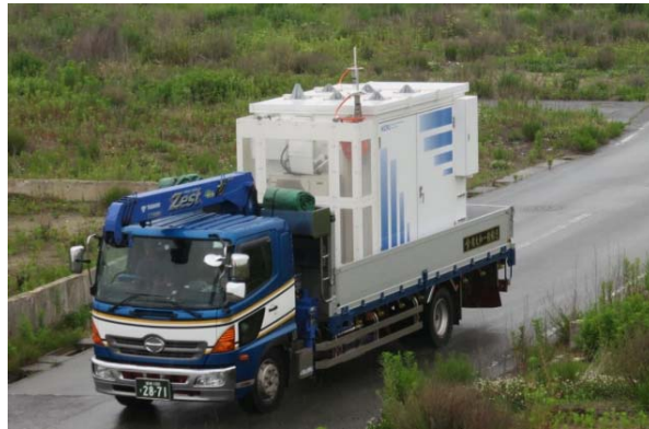
Figure 5.2: Transporting an MDRU to a Remote Disaster Site (ITU, 2015)
