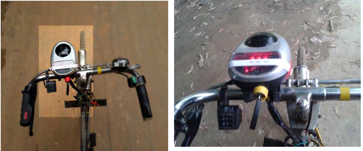
Fig: Power Key and charge indicator
