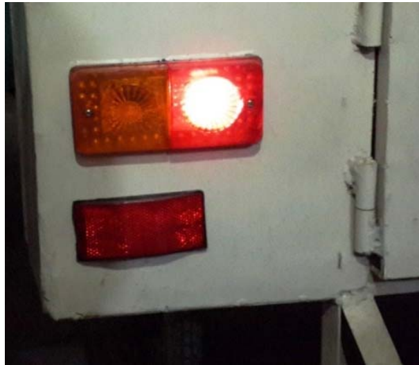
Fig. 2.20 Brake light is on
