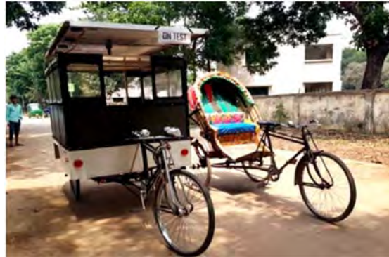
Fig. 1.3 Modernized Rickshaw-van (left), Traditional Rickshaw (right)
