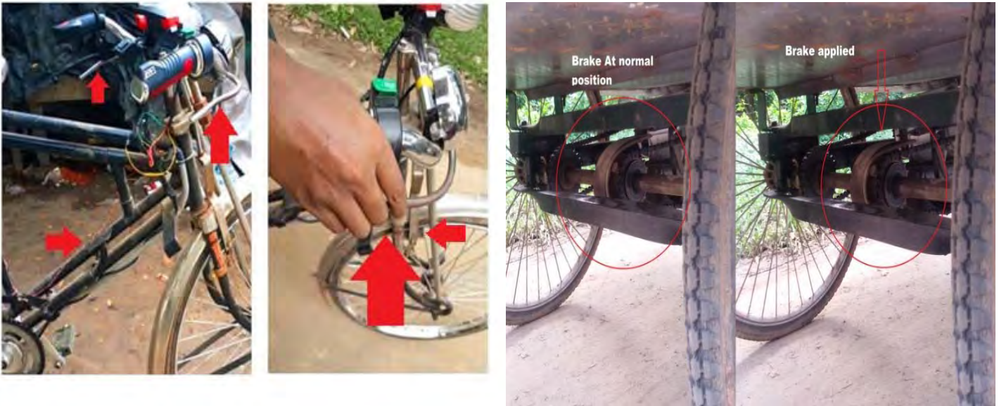
Fig: Hand-clutch and rear wheel brake pedal
