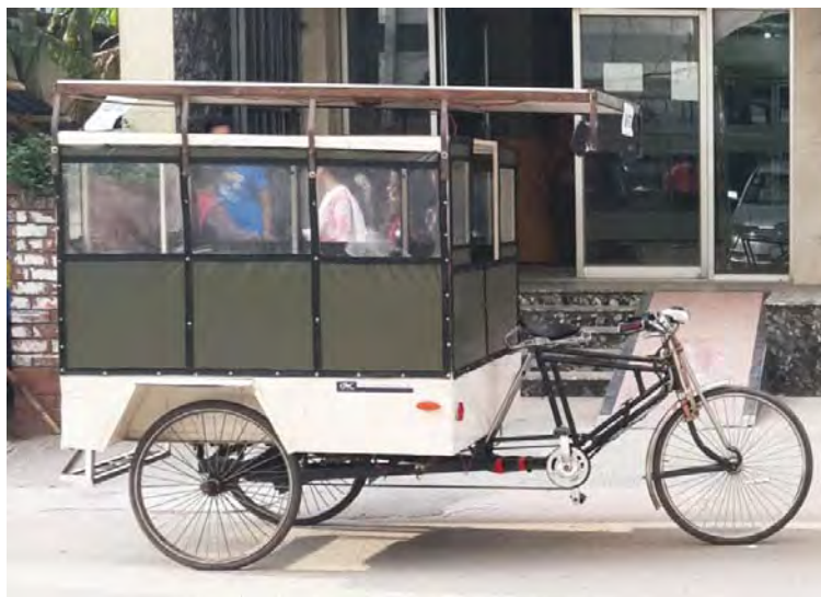
Fig 3.5 Rickshaw-van with torque sensor pedal and PV support
