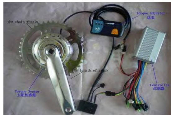
Fig. 4.1 Complete set-view of torque sensor and other components [16]
