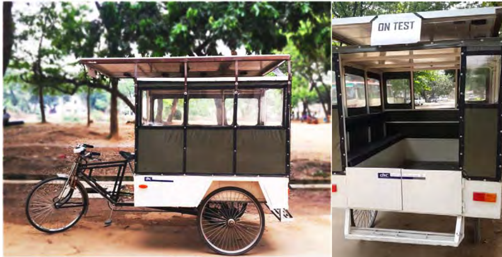
Fig.6.1 Side and rear view of solar tri-wheeler
