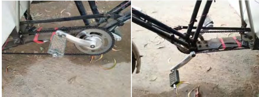
Fig. 4.3 The torque-sensor pedal
