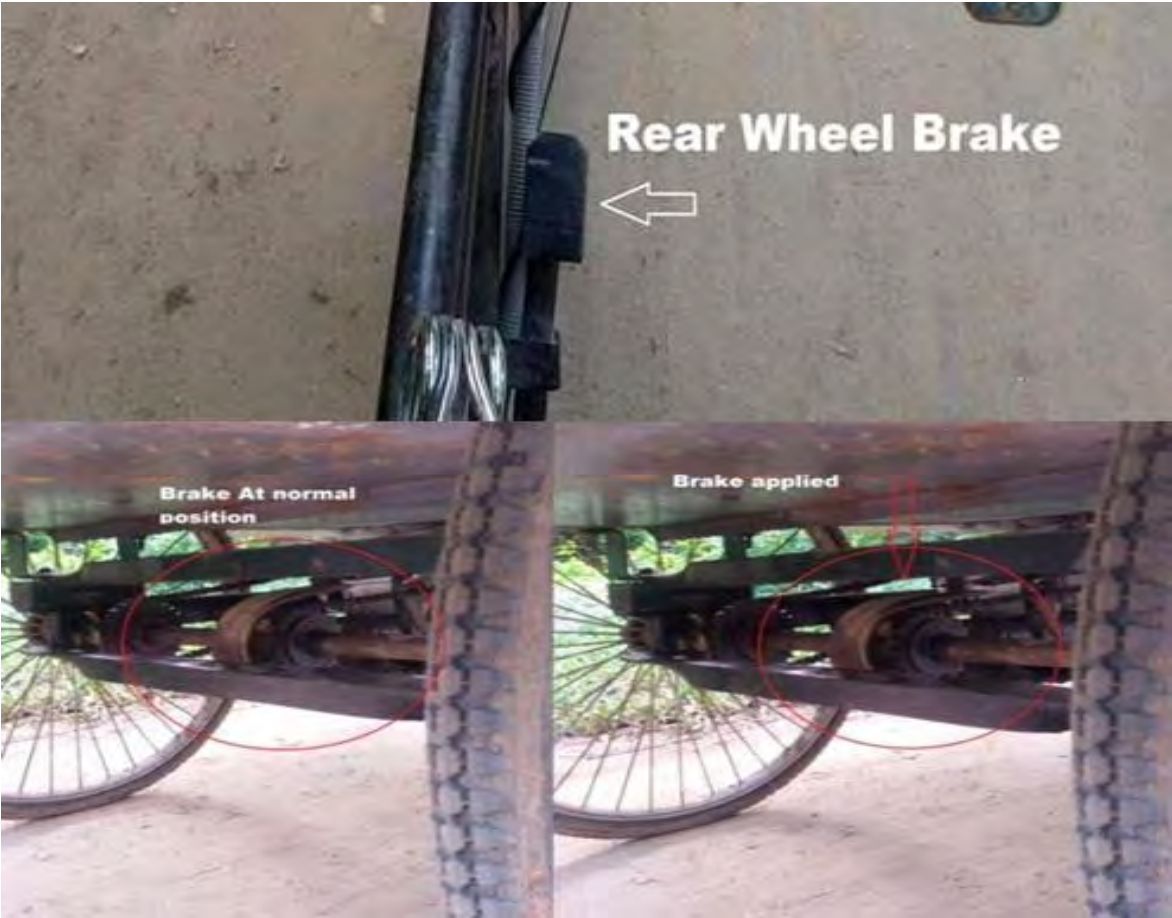
Fig. 2.15 Rear wheel brake
