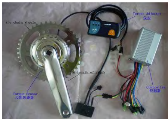
Fig. 4.1 Complete set-view of torque sensor and other components [16]
