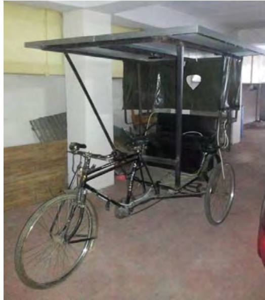
Fig 3.4 Electric rickshaw with PV panel installed in “flat state”
