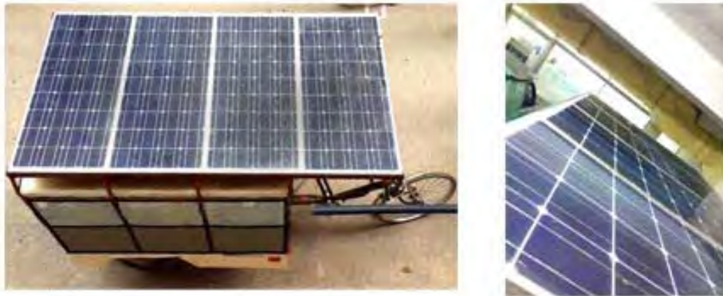
Fig. 4.9 Solar panel on rickshaw -van
