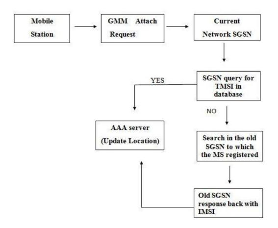
Fig.5.1 Block Diagram for UMTS Entry Process
