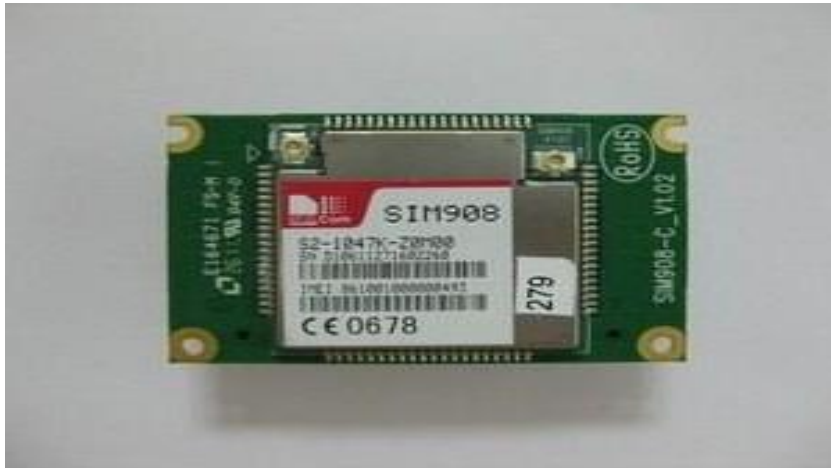
FIGURE: 4.1.E-SIM908 Module
