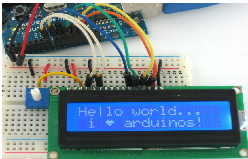
Fig 1.10 : LCD connected with Arduino
