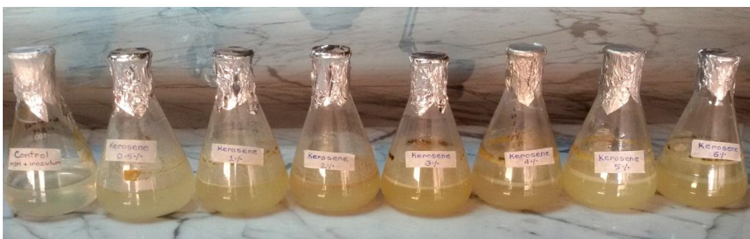
Figure 3.2.1: Growth of C1 isolate in mineral salts broth containing varying concentrations of kerosene. After 7 days incubation at 35°C and 120 rpm, the broth turned turbid due to growth of the microbe. Turbidity was observed to gradually increase, showing maximum turbidity at 3% kerosene, and again decline at concentrations higher than 3% kerosene.
