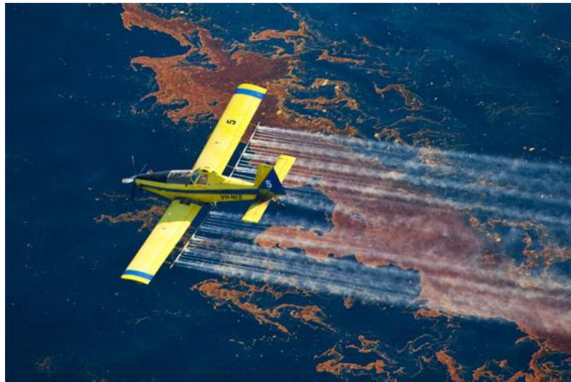
Figure 1.7: Current chemical removal of oil pollutants include the spraying of carcinogenic dispersants (Montara Well Head Platform, 2009)
