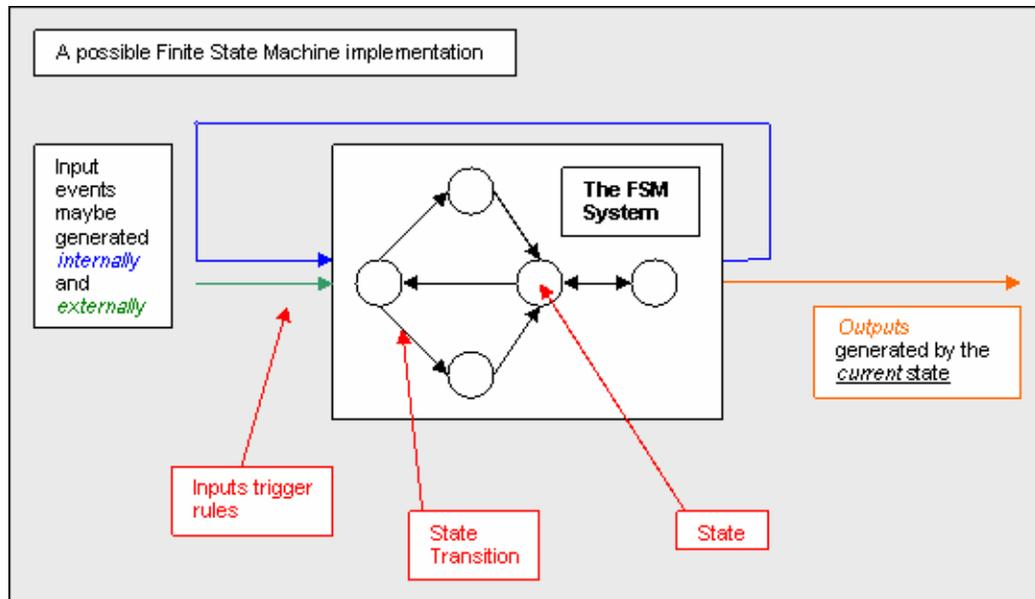
figure 1.1: A possible finite state machine implementation
