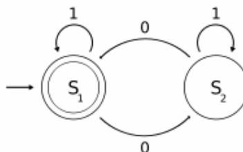
An example of an accepting state appears on the left in this diagram of a deterministic finite automaton which determines if the binary input contains an even number of 0s. S1 (which is also the start state) indicates the state at which an even number of 0s has been input and is therefore defined as an accepting state.
