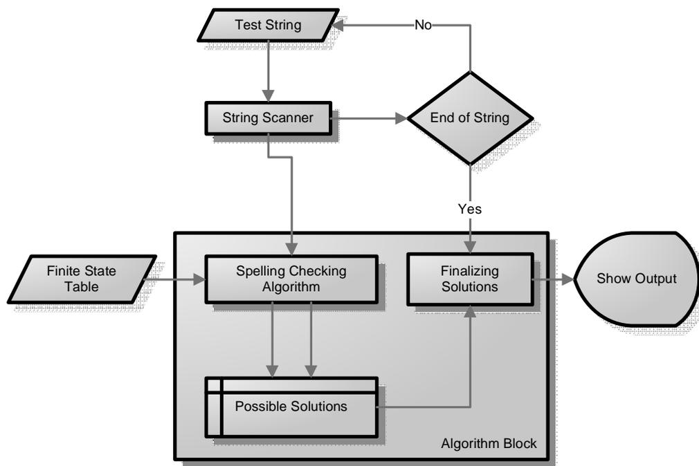
figure 2.2: Spelling Checker System Block Diagram
