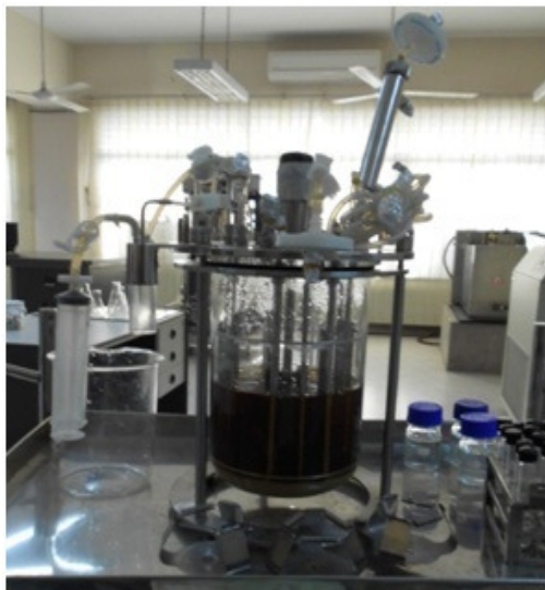
Figure 2.3: Preparation of Bioreactor for autoclaving
