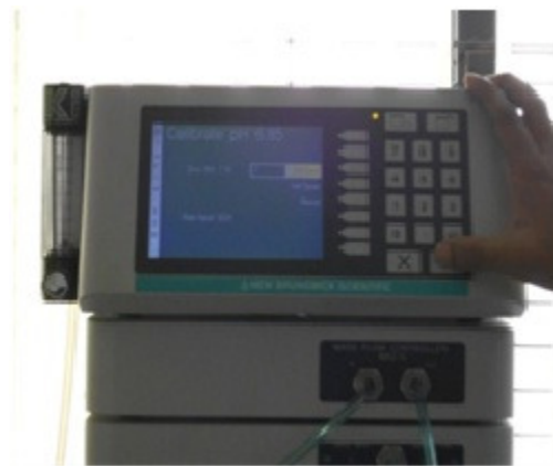
Figure 2.5: pH probe was calibrated before autoclaving
