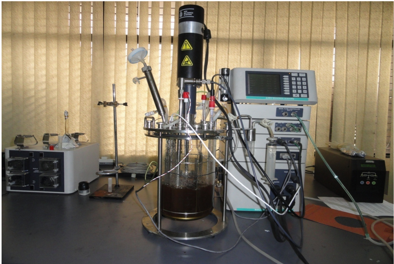
Figure 2.2: BIO FLO 110 Bioreactor; NEW BRUNSWICK SCIENTIFIC
