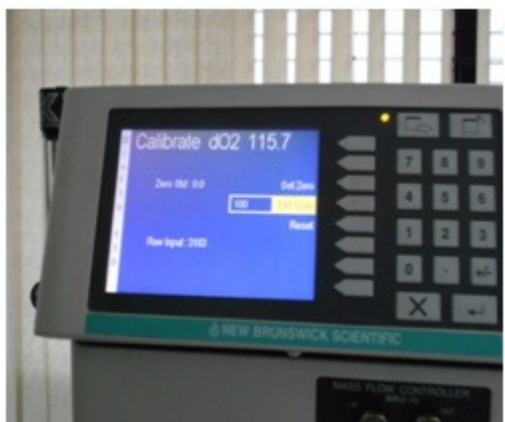
Figure 2.4: dO_2 probe was calibrated after autoclaving
