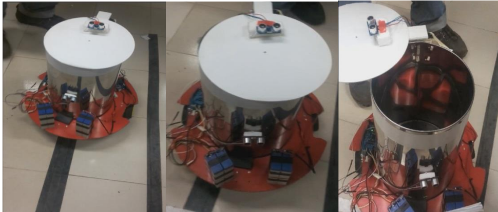
Figure 10: Path Following with Bin Cover opened & closed
