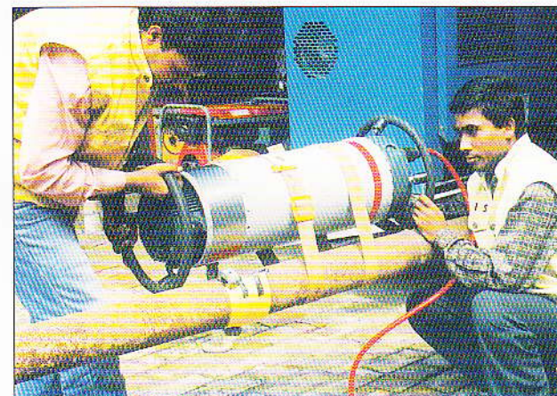
Radiography of WOT using X-Ray at our workshop
