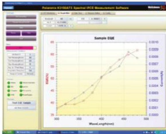
Figure 16 Ideal cell EQE output against wavelength and current [4].
