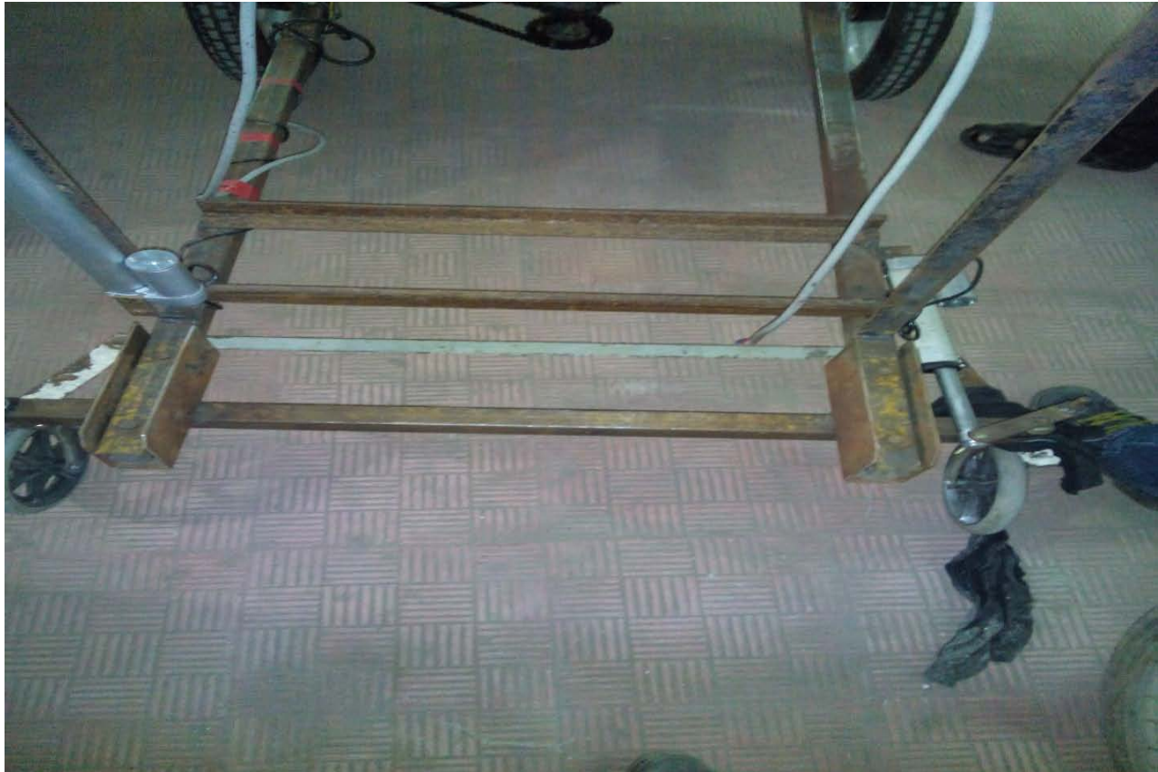
Figure 7: Ackerman Steering Wheels with Linear Actuator attached sideways
