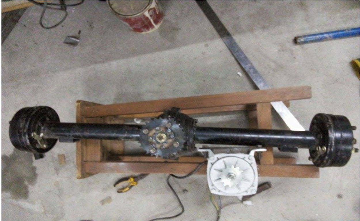
Figure 3: Actual diagram of Differential mounted with 48V Brushless DC motor
