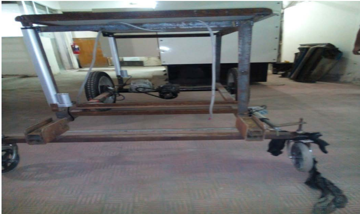
Figure 10: Position of Linear Actuators during Loading Goods
