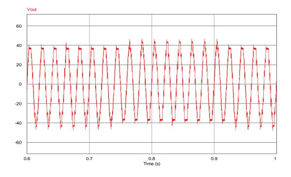
Figure 5.4.1: Output after using LPF
