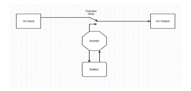
Figure 2.3: Standby power Supply
