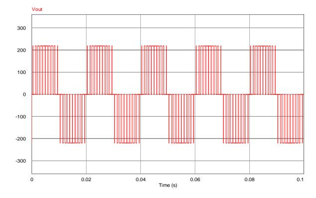
3.5.2 Output waveform for PWM inverter (Unipolar):
