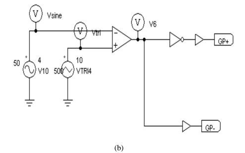
Figure 3.6: Bipolar PWM inverter circuit (a), gate pulse (GP+) for sw14 (b), gate pulse(GP-) for sw23(b)
