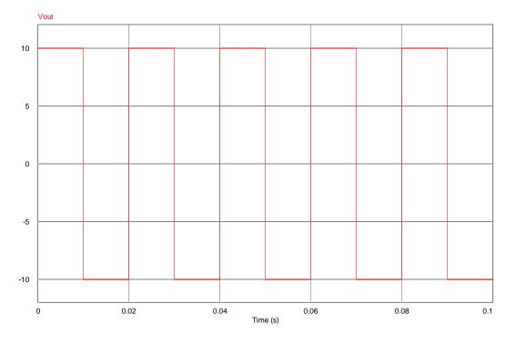
Figure 3.1.3: Output waveform of square wave inverter
