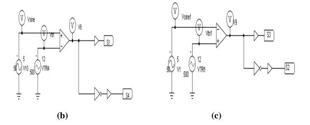
Figure 3.12: Unipolar PWM inverter (a), gate pulse for sw14 (b), gate pulse for sw23 (b)
