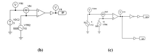
Figure 5.1: Integration of Boost converter and Inverter circuit (a), gate pulse for sw (b), gate pulse (gp+) for sw2 and gate pulse (gp-) for sw3 (c)
