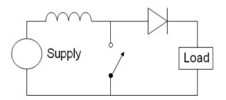
Figure 4.1: Basic schematic of boost converter
