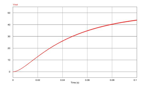
Figure 4.2.3: Output waveform of boost converter
