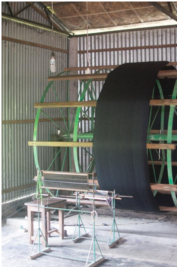
Fig 16: Thread Warping machine present in Pathrail, Tangail
