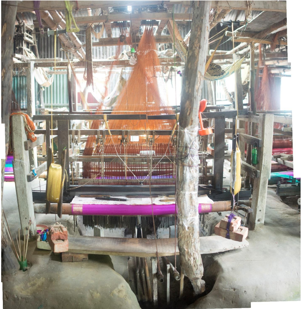
Fig 15: Traditional Pit-loom machine with Jacquard Weaving
