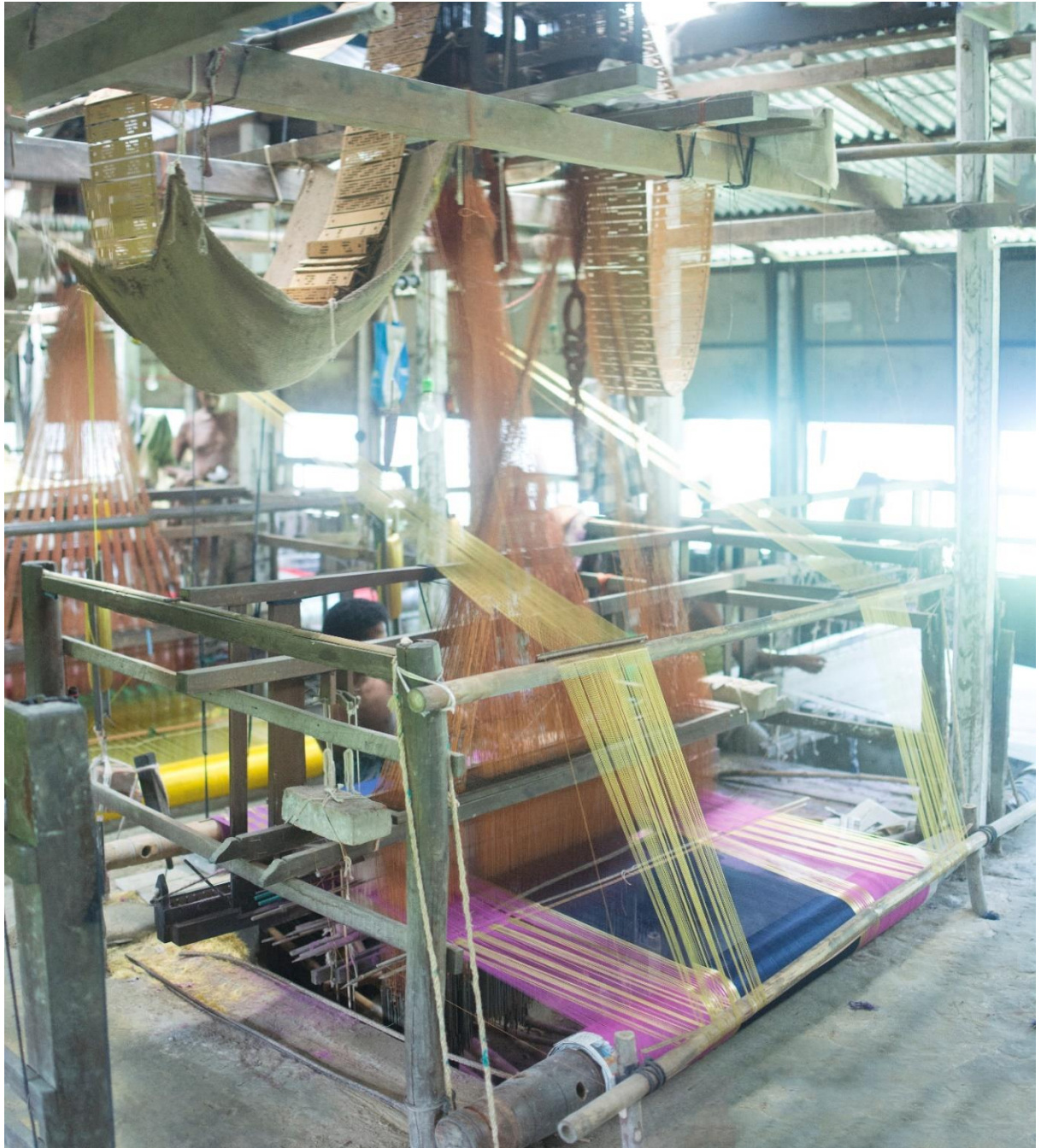
Fig 14: Traditional Pit-loom machine with Jacquard Weaving
