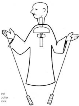
Fig 3.4.2.3 A central control rod with a supporting collar to hold the shoulder block permits turning [Currell, 1999].
