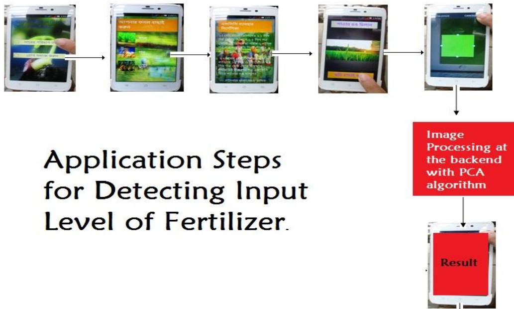
Figure 5: Steps of detecting input level of fertilizer
