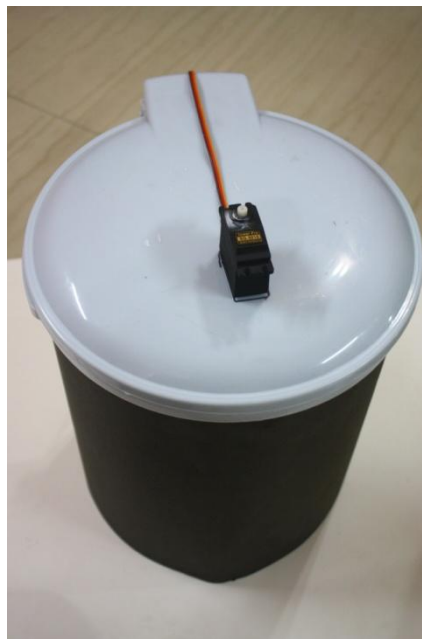
Figure 6: Servo motor on top for ultrasonic sensor movement.
