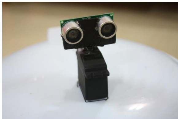
Figure 7: Ultrasonic sensor mounted on servo motor.
