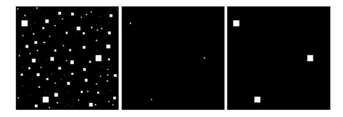
There could be gap in between congested pixel, that could hamper in counting vehicle. For smooth counting and perfect blobbing dilation is mandatory. Erosion and dilation both process comes in a series. From diagram after erosion in fig 2 contains less noise then fig 1. After Erosion for perfect blobbing we do dilation, blobs is more accurate and well shaped for counting.
