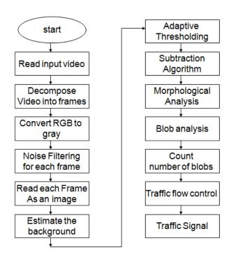
Applying background subtraction algorithm with noise Reduction process we find the the number of vehicles in the road .Number of blobs is the actual density of vehicle .Number of blobs is a int value and for number of vehicle on road Traffic light and signal changes. I implemented my project on hardware with arduino. Traffic lights Red, Green and Yellow changes for traffic density to control the flow of traffic On road.
