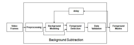
There are a several approaches in background subtraction for static and dynamic background. Based on requirement researcher used those algorithm among them Frame difference , Adaptive background Subtraction ,Gaussian Mixture , kernel density estimation are well known . Every algorithm has positive and negative impacts , some takes much computation time others are good for less noise and dynamic model.
