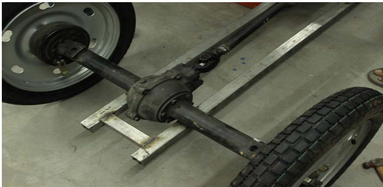
FIGURE 9.5.1: REAR AXLE OF THE CAR (initial state of chassis)
