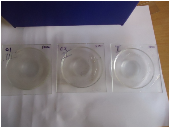
Figure 4.5: a) Sugar estimation by DNS method, b) After 24 hours fermentation in shaking condition, c) Conway unit used for Ethanol detection
