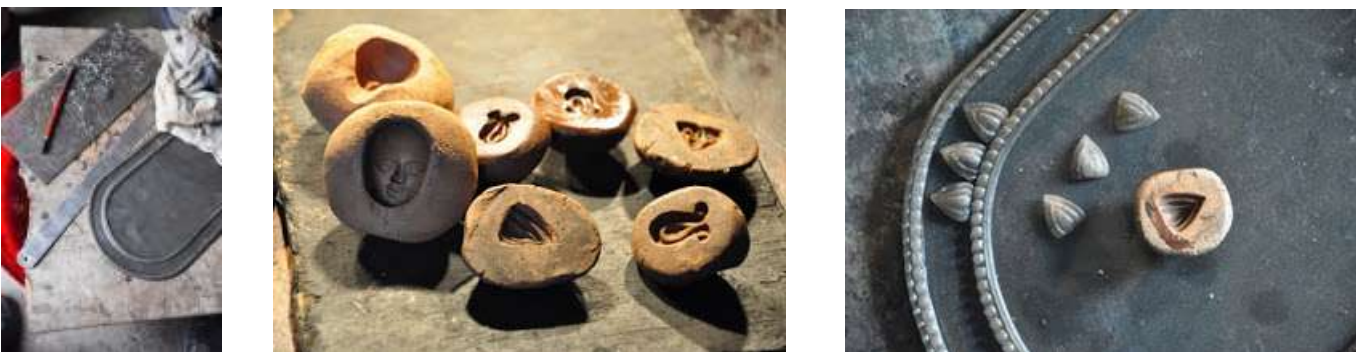
Figure 3.7.1.3 a: Sprig moulds for lost wax method (Source: Dhamrai Metal casting, Making Space: Sensing Place, Steven Follen)
