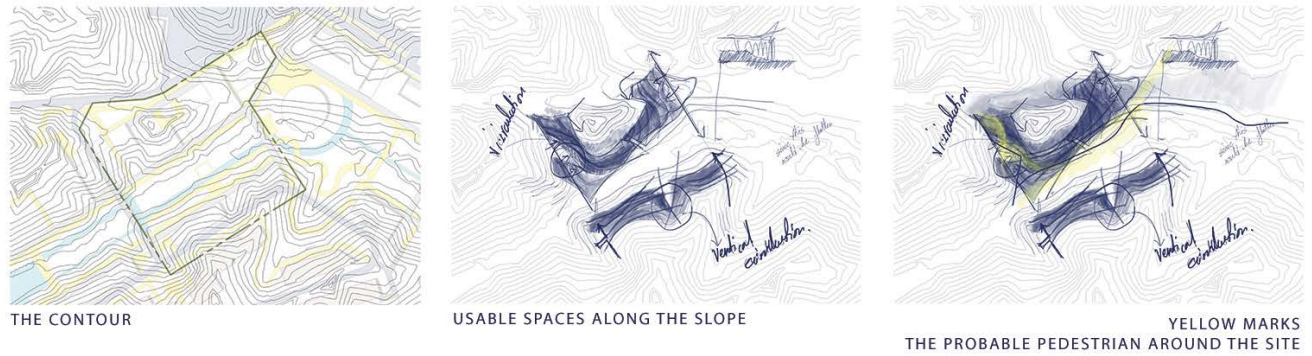
Fig: 19 Analysing the usable areas on the slope of terrain, source: author
