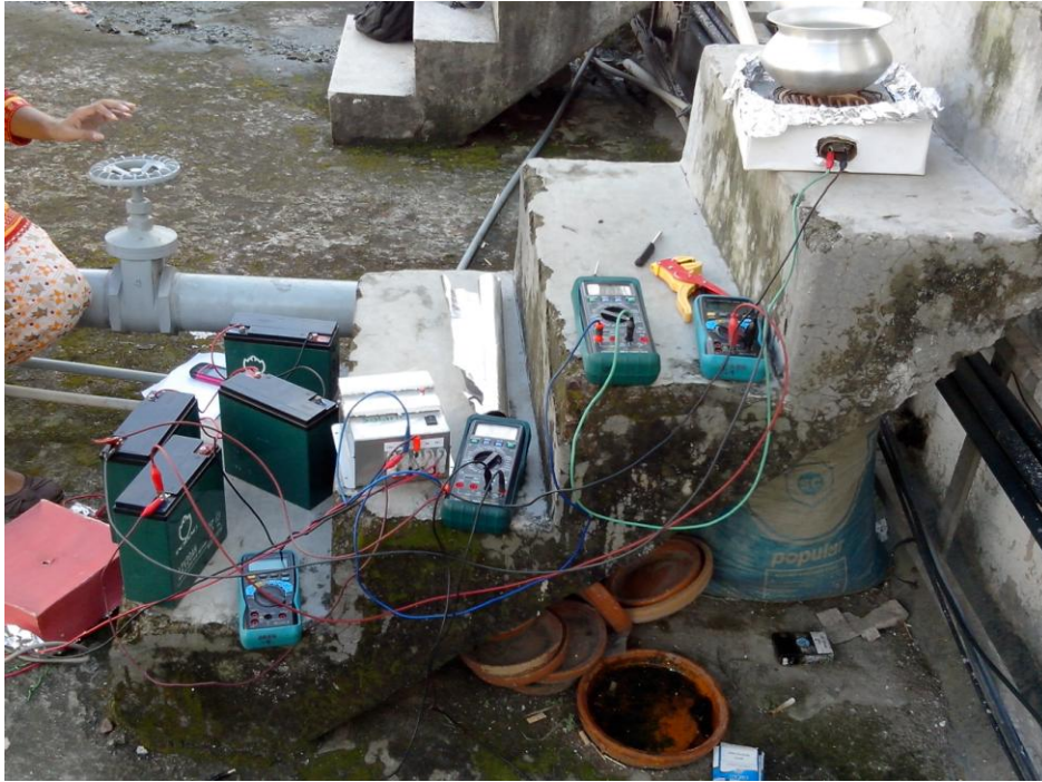
Fig 2.9 Battery discharging by load through controller
