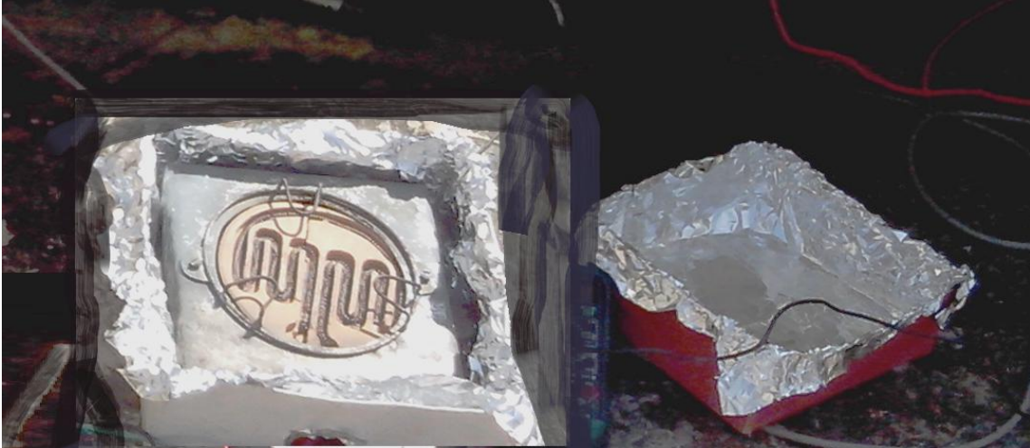
Fig 4.2: Electric stove covered with aluminum foil paper(heat insulator)
