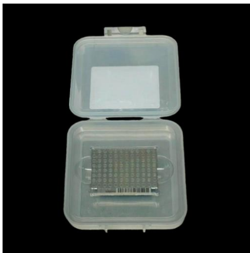
Figure 2.9.1 : Matrix plate (MSP 96 target)
