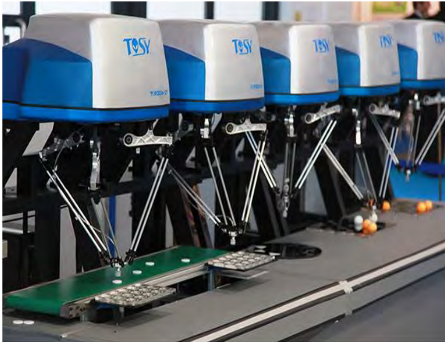
Figure 3: The robotic linkage arm is used in electronics production lines with the lighting effect.
