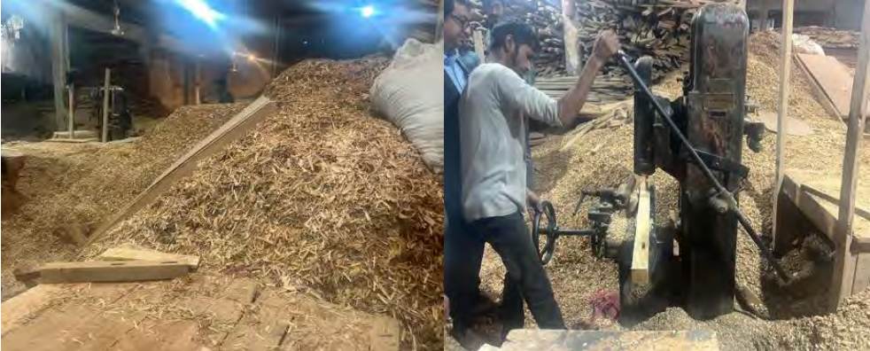
Fig 28: Wood dust causes machinery to deteriorate and health hazard (Source: BFIDC).
