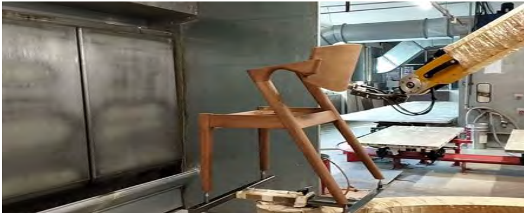
Fig 1: A robotic arm applying lacquer polish to a chair at HATIL factory (Source: HATIL).
