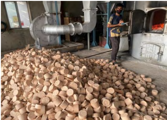
Fig 23: Compressed blocks (briquettes) made from dust Fig 24: Thermo fluid heaters
